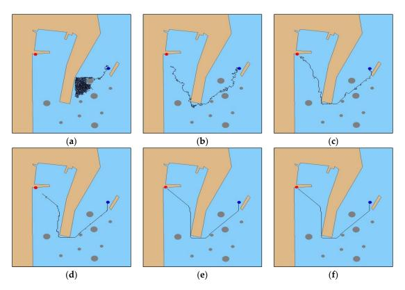
**Figure 8.** Improved DRL algorithm to verify the experimental results: (**a**) initial iteration; (**b**) 100th iteration, (**c**) 500th iteration, (**d**) 1000th iteration, (**e**) 1500th iteration, and (**f**) 2000th iteration.
