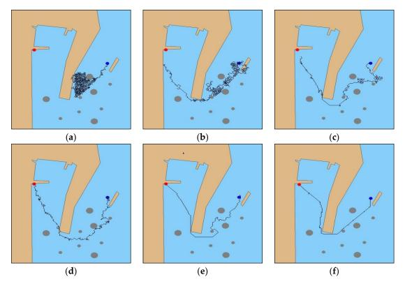
**Figure 7.** DRL algorithm verification experiment results: (**a**) initial iteration; (**b**) 100th iteration, (**c**) 200th iteration, (**d**) 500th iteration, (**e**) 1000th iteration, and (**f**) 2000th iteration.
