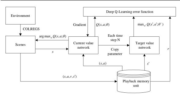
Figure 5. Main flowchart of the autonomous navigation decision-making for MASS.
