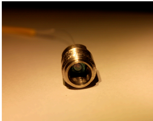
Figure 7. The fiber-optic pressure sensor with a full SiC sensor head.
