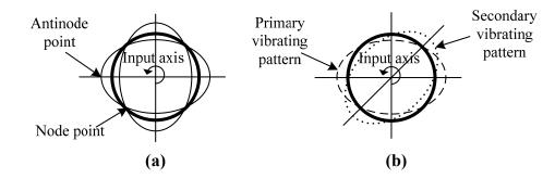
The math model proposed by Lynch is used in this paper with the resonator operating in the  $n = 2 \mod [17,18]$ . In the math model, mass and stiffness imperfections causing frequency split between the two modes and inhomogeneous damping dependent on the circumference angle are considered. The equations are presented as follows:
