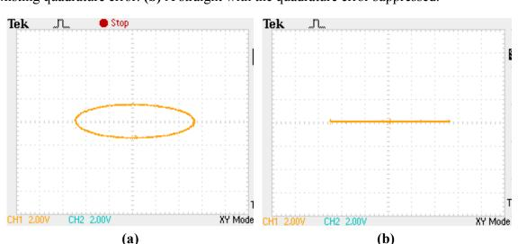
**Figure 2.** Lissajous figure on two electrodes with an angle distance by 45°. (a) An ellipse existing quadrature error. (b) A straight with the quadrature error suppressed.
