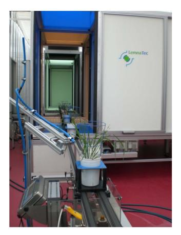
Figure 2. Barley plants at the weighing and watering unit after leaving the imaging station.
