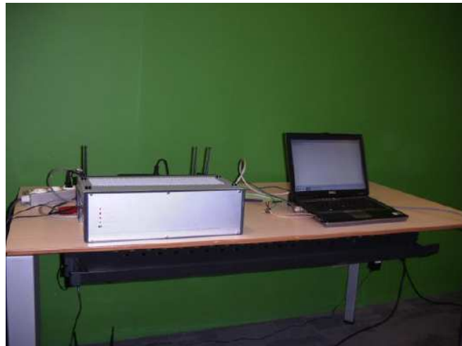
Figure 23. Philips WSD cognitive radio node.
