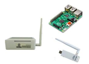
Figure 4. Listening device used in the people flow monitoring sensor network.
