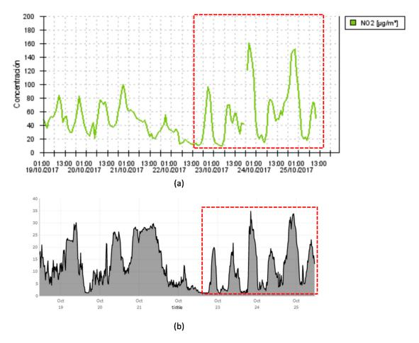
**Figure 17.** (a) NO<sub>2</sub> concentration measured by a municipal air quality monitoring station [51]; (b) NO<sub>2</sub> concentration measured by the outdoor environmental sensor of the Industrial Engineering School, which is in front of the municipal monitoring station.
