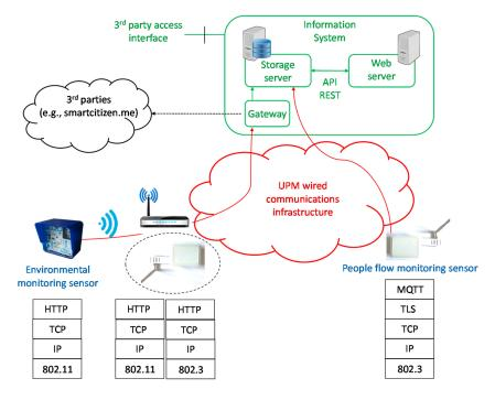
**Figure 9.** Overview of the communications architecture and protocol stack of the Smart CEI Moncloa platform.
