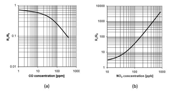
Figure 7. MiCS-4514 calibration curves: (a) CO concentration; (b) NO<sub>2</sub> concentration [30].
