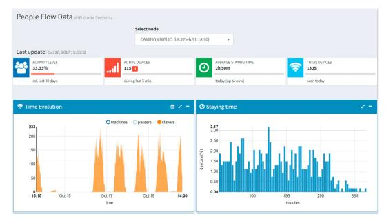
**Figure 11.** View associated to the people flow monitoring sensor installed in the library of the Civil Engineering School.
