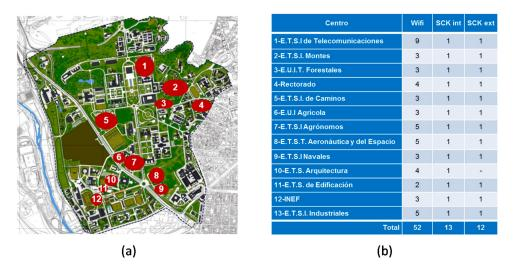
**Figure 5.** Summary of the sensors deployed in the Smart CEI Moncloa (November 2017): (**a**) Location of the schools within the Campus; (**b**) number and type of sensors per site.
