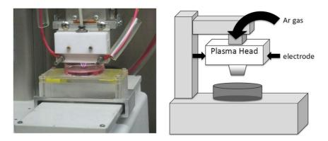
Figure 1. Scheme of generation of nonequilibrium atmospheric pressure plasma (NEAPP)-activated medium. doi:10.1371/journal.pone.0081576.g001
