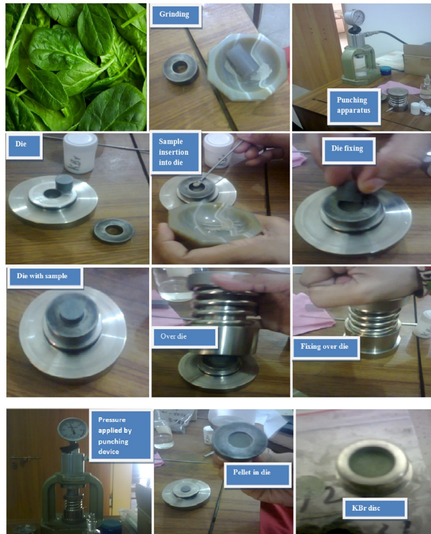
Fig 1. Procedure of Fourier Transform Infrared Spectroscopy usage for analysis of samples. Each subsection picture is showing the step involved in the analysis.
