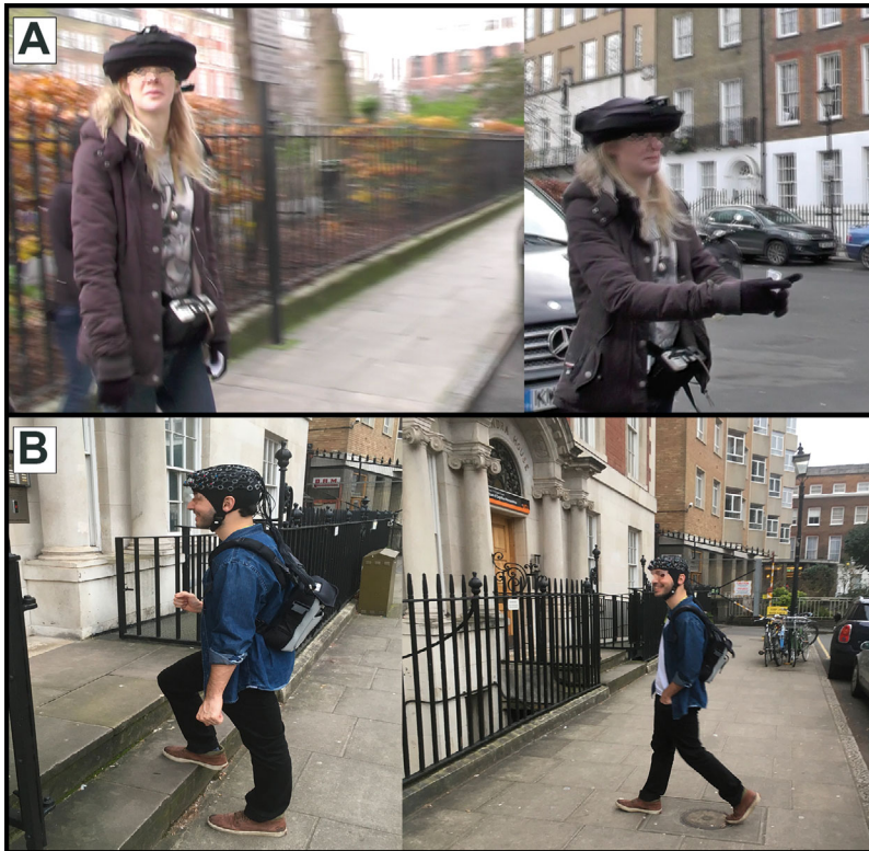
Figure 7. (A) Example of a participant carrying out the ecological prospective memory task described in Ref. 60 in the real world where brain activity is monitored over the PFC by a portable, wearable, and fibreless fNIRS system (WOT-100, Hitachi, Japan; now sold by NeU Corporation, Japan). (B) Example of a participant freely moving in unrestrained situations outside the lab while functional brain activity is measured over the PFC through a portable and wearable fNIRS device (LIGHTNIRS, Shimadzu, Japan); such system is equipped with optical fibers that are connected to a control unit, carried through a backpack.
