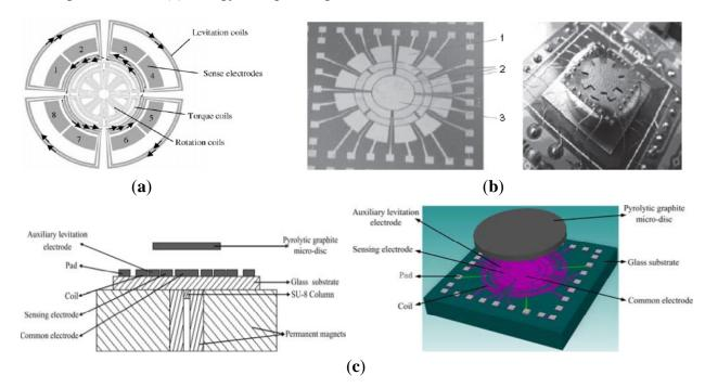
**Figure 17.** (a) University of Electronic Science and Technology suspended rotor gyroscope. (b) Schematic diagram of magnetic actuator.
