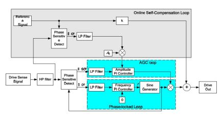
Figure 40. Scale factor compensation.
