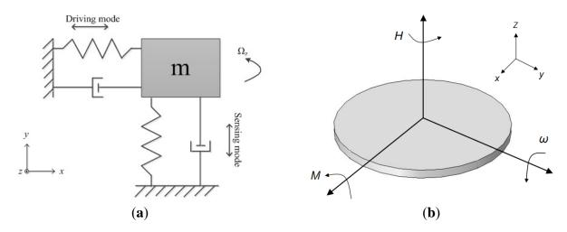
The conservation of angular momentum is shown in Figure 1b. The micromachined gyroscope based on precession principle usually has a rotor which is rotating around the spin axis (z-axis) at a constant speed to maintain an angular momentum  $\mathbf{H}$ . When an angular rate orthogonal to the spin axis is applied, such as around y-axis, a precession moment  $\mathbf{M}$  of the rotor is generated around x-axis by the equation:
