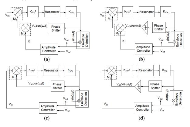
Figure 28a,b are the AC amplitude control loops. The phase shifter (PS) is used to match the resonant frequency, and the signal after amplitude detection is used to control the AC amplitude of the excitation signal in the amplitude controller. M<sub>2</sub> is a multiplier used as a variable-gain amplifier (VGA) to control the amplitude of AC signal. M1 is the multiplier to multiply the AC and DC signals
