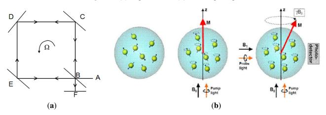
The principle of nuclear magnetic resonance gyroscopes (NMRGs) is to measure a corresponding shift in the Larmor precession frequency where the nuclear spins is applied in magnetic field. As shown in Figure 2b, when a static magnetic field  $B_0$  is applied, the magnetic moments will rotate about the direction of  $B_0$  at the Larmor precession frequency  $\omega_L$ :
