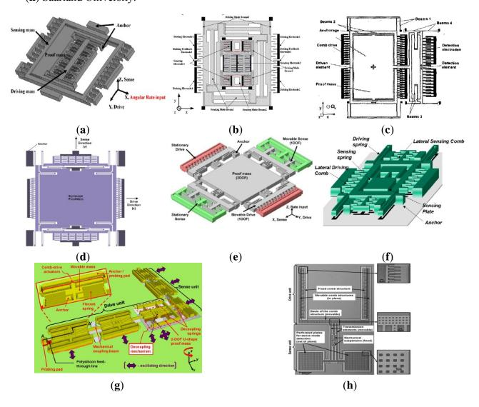
Figure 4c shows the doubly decoupled gyroscope of HSG-IMIT [32]. This gyroscope comprises four types of springs (beams 1 to beams 4) and three oscillators. Due to the arrangement of the springs, only the driven element and the proof mass are excited to a linear oscillation along the drive mode (x-
