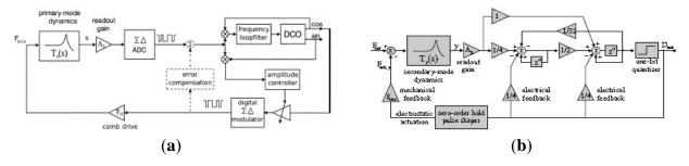
In [182], an optimal unconstrained architecture for such force-feedback loop was presented. Considering the mixed electrical and mechanical systems, an electrical resonator which is built by
