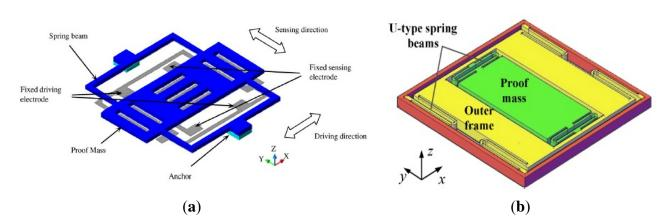
Figure 23. Slot-structure gyroscopes. (a) SIMIT. (b) Zhejiang University.
