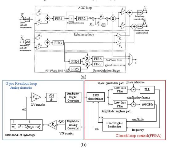
Figure 33. FPGA circuits. (a) JPL. (b) PKU.
