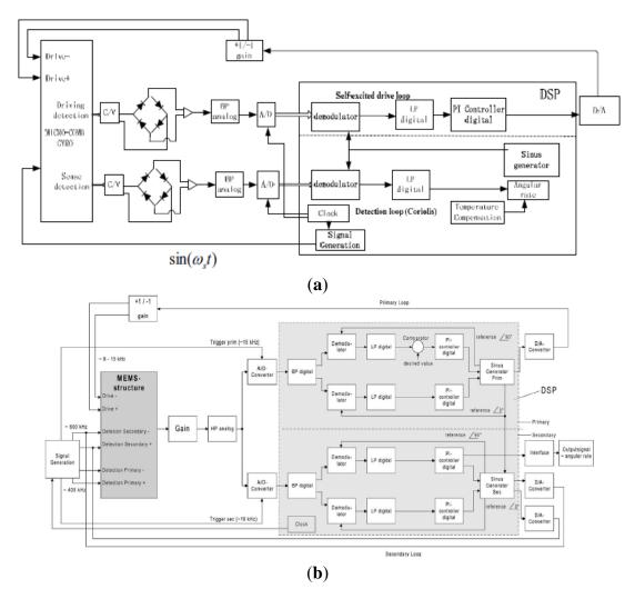
Figure 32. DSP circuits of (a) PKU. (b) HSG-IMIT.
