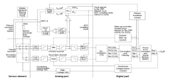
**Figure 35.** Gyroscope circuitry of Helsinki University of Technology.
