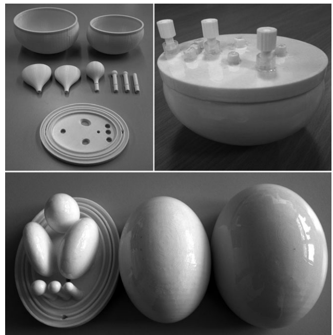
FIG. 4. MRI 3D printed phantom. 58 Figure license: Kasten, et al., 2016, 3D-printed Shepp-Logan phantom as a real-world benchmark for MRI. Copyright maintained by John Wiley and sons, all rights reserved.
