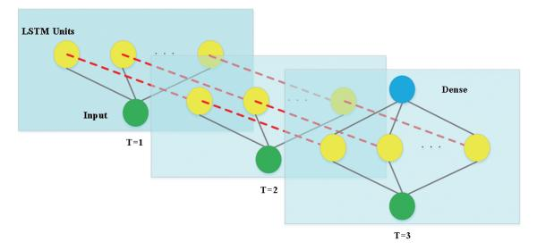
**Figure S7** LSTM network structure used. Input was a fixed time step data. This model used three days of new infections as input, input dimension (3,1). The Hidden Layer received input data from the Input Layer into the middle tier of the LSTM unit, set to 25. The Dense Layer received inputs from the output vector of the Middle Layer of the LSTM into the full-connection layer, from which the output was the final regression result. LSTM, Long-Short-Term-Memory.
