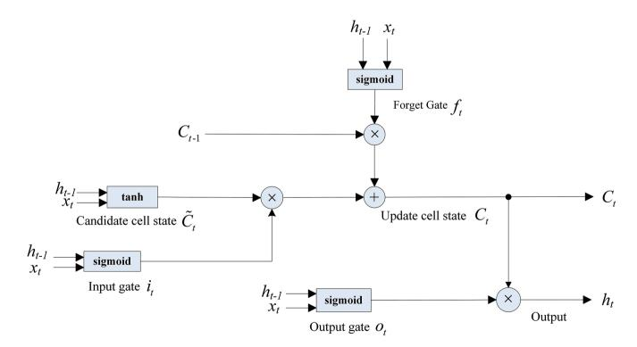
Figure S6 LSTM inner structure. LSTM, Long-Short-Term-Memory.
