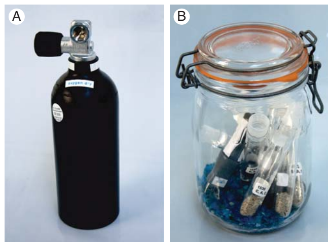
FIG. 1. Storage containers used in the experiments. (A) Steel tank with an internal volume of 1.5 L which can be filled with gas to 20 MPa pressure. (B) Glass jar containing air at ambient pressure (0.1 MPa), showing the perforated tubes with seed samples, silica gel for RH buffering and a data logger for recording RH and temperature.
