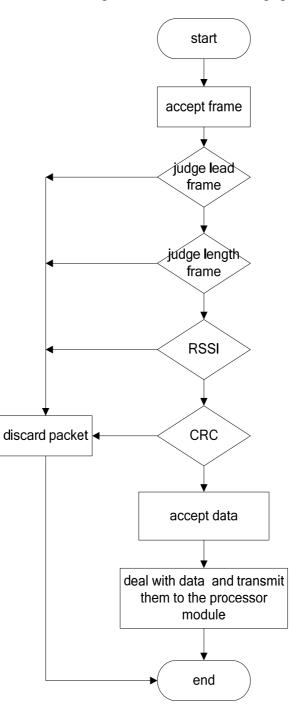
Figure 9. The flow diagram of the CC2420 accept process.
