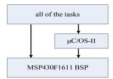
Figure 16. MSP430 module software level diagram.
