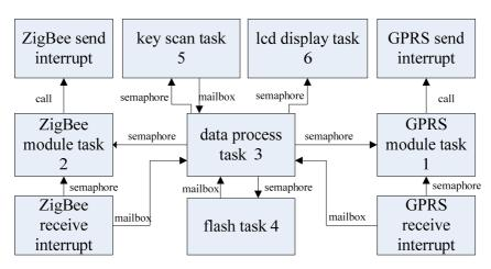
Figure 17. The communication diagram of each task.
