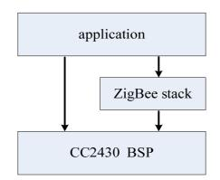
Figure 14. ZigBee module software level diagram.
