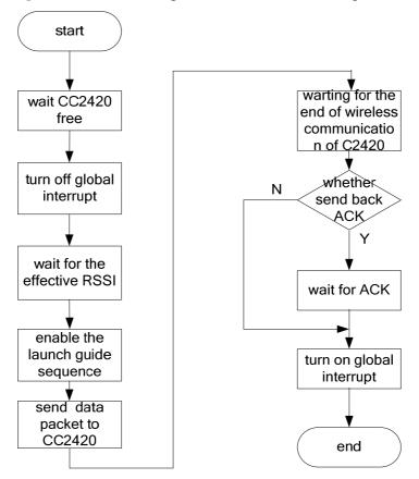
Figure 8. The flow diagram of the CC2420 send process.
