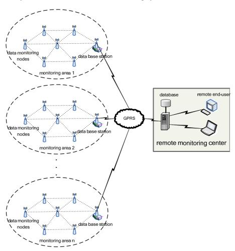
Figure 1. Water environment monitoring system based on WSNs.
