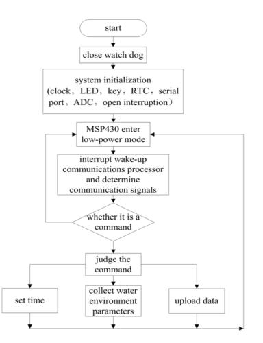
Figure 7. The flow diagram of the master routine.
