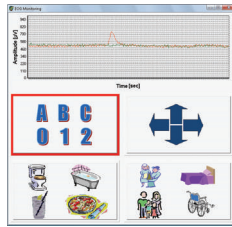
(c) User interface main menu. At the top line horizontal and vertical EOG signals can be observed online. The other options for virtual keyboard, needs, and movement control can be selected
