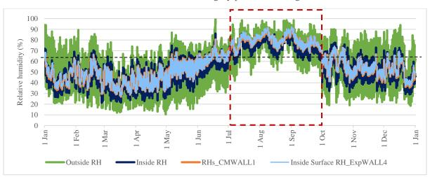
Figure 12 Varying RH levels with time throughout the year in PT\_B.
