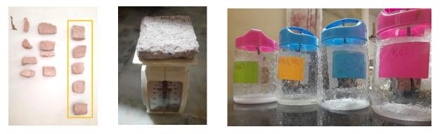
Figure 7 Lime plaster samples for the experiment Figure 6 Four jars containing different salt solutions.
