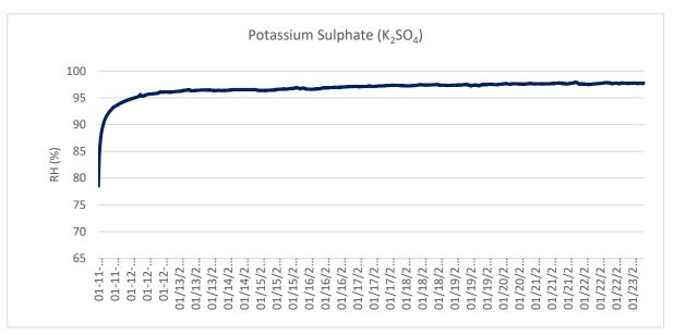
Figure 54 96% RH maintained by K<sub>2</sub>SO<sub>4</sub>
