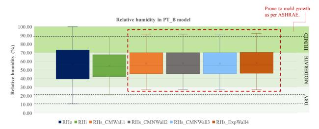
Figure 11 Relative Humidity levels of space and on the surface of the walls in PT\_B.
