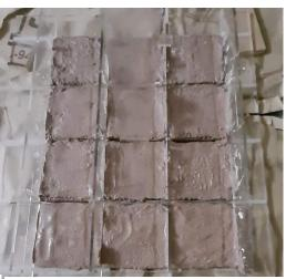
Figure 57 Lime Plaster samples in a battery mold for curing.
