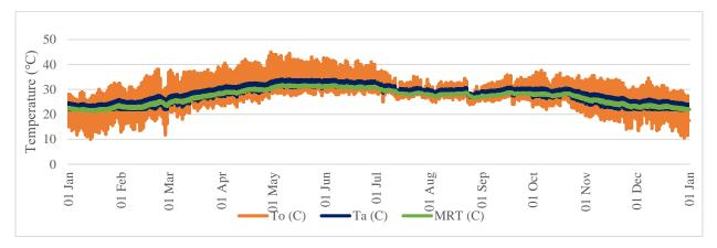
Figure 10 Simulations results showing a range of outdoor, indoor, and mean radiant temperature in PT\_B.
