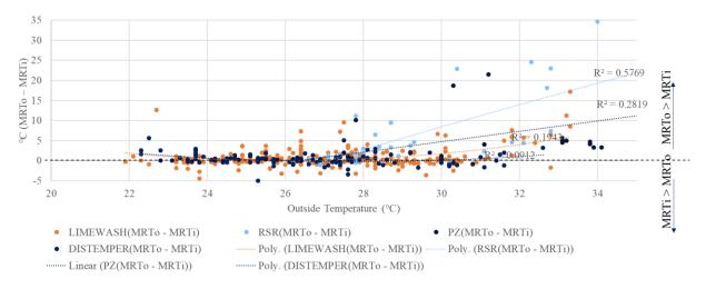
Figure 24 MRT performance for different categories of lime plaster survey cases.
