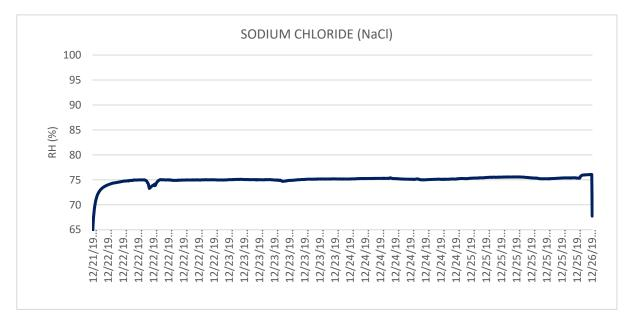
Figure 52 75% RH maintained by NaCl
