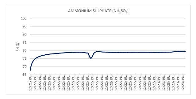
Figure 53 80% RH maintained by NH<sub>2</sub>SO<sub>4</sub>
