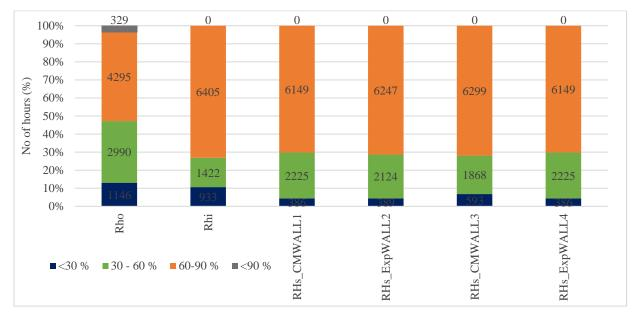
Figure 16 PS\_A RH levels observed throughout the year with respect to the number of hours.
