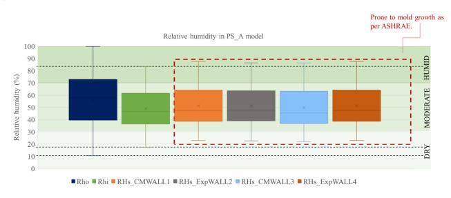
Figure 14 Relative Humidity levels of space and on the surface of the walls in PS\_A.
