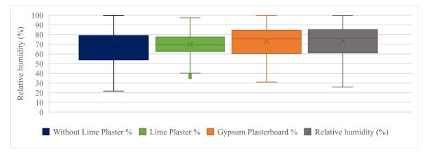
Figure 9 Indoor Relative Humidity for different cases.
