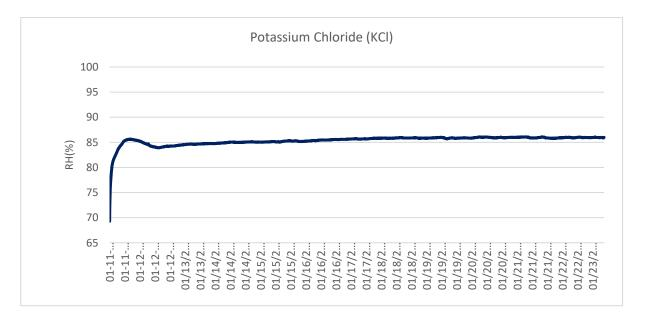
Figure 55 86% RH maintained by KCl
