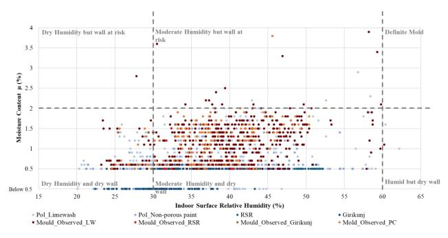
Figure 29 Moisture content Vs Surface relative humidity
