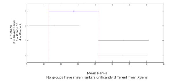
**Figure 6.** Kruskal–Wallis test result for Xsens roll and pitch RMS compared to Galaxy Nexus, iPhone 5S and iPhone 4 for the dynamic protocol at rate of 50% of the maximum velocity.
