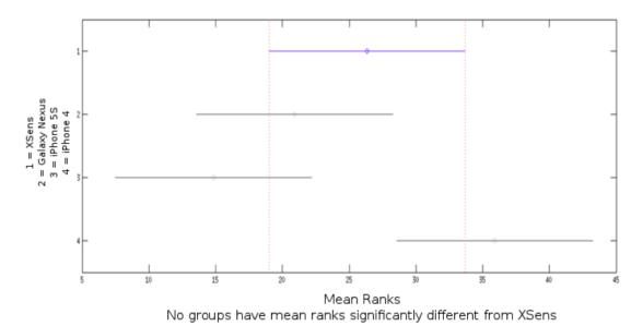
**Figure 5.** Kruskal–Wallis test result for Xsens roll and pitch Root Mean Square (RMS) compared to Galaxy Nexus, iPhone 5S and iPhone 4 obtained for the static protocol.
