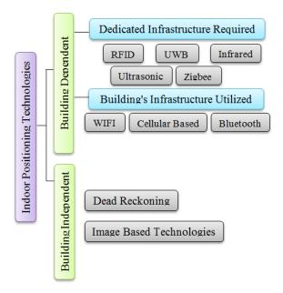
Figure 3. Classification of indoor positioning technologies.
