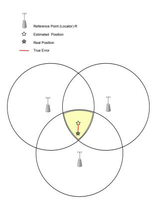
Figure 1. Positioning using reference points.
