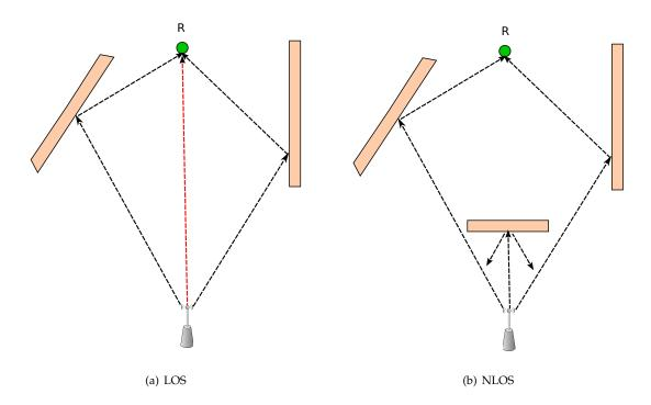
Figure 2. (a) Line-of-sight (LOS) vs. (b) non-line-of-sight (NLOS).
