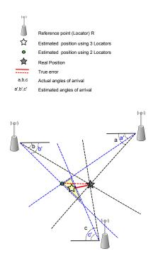
Figure 4. Angle of arrival (AOA)-based algorithms.
