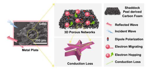
Fig. 6 Schematic illustration of microwave absorption mechanisms for 3D shaddock peel-derived carbon aerogel
