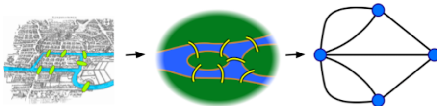
Figure 1: Euler abstracted the problem to a set of nodes and edges and launched network theory.
