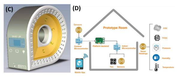
**Figure 4.** Illustration of the proposed electronics nose (E-nose) system architecture (**A**); the proposed E-nose application in future smart buildings (**B**); primitive concept design of Smart-Air (**C**); and a smart ventilation system for optimizing indoor air quality (IAQ) Levels in buildings (**D**). Reproduced with permission from [180,181,183,184].
