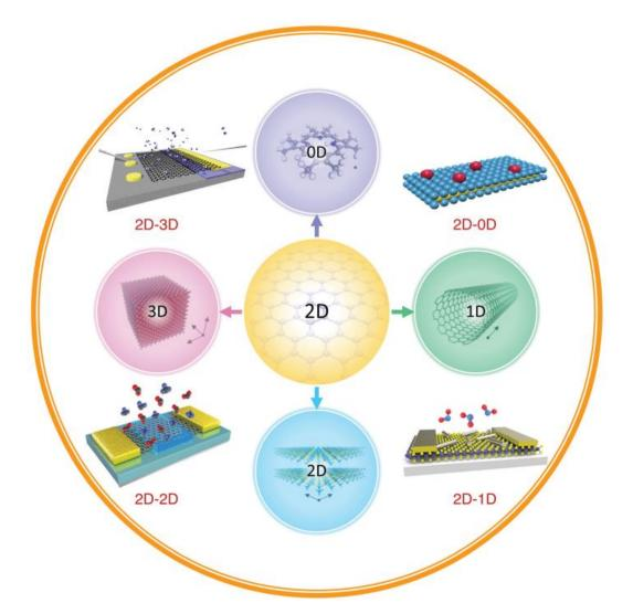
**Figure 3.** Schematic overview of 2-D nanostructured materials and different types of heterostructures with 0-D, 1-D, 2D, and 3-D materials used for gas-sensing applications. Reproduced with permission from [164].
