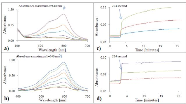
**Figure 3.** FRAP absorption spectra (450 – 700 nm) for gallic acid (**a**) and  $\text{Trolox}^{\mathbb{R}}$  (**b**). Dependence of absorbance of FRAP with gallic acid (**c**) and  $\text{Trolox}^{\mathbb{R}}$  (**d**) on time.
