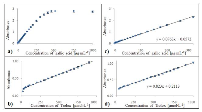
**Figure 10.** Dependences of absorbance of colour product on concentration of gallic acid (a) and  $\text{Trolox}^{\text{(B)}}$  (b). Calibration curves for DMPD method related to equivalent of gallic acid (c) and  $\text{Trolox}^{\text{(B)}}$  (d) expressed in units of absorbance.
