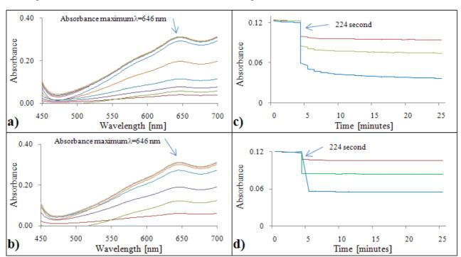
**Figure 2.** ABTS absorption spectra (450 – 700 nm) for gallic acid (**a**) and  $\text{Trolox}^{\mathbb{R}}$  (**b**). Dependence of absorbance of ABTS radical with gallic acid (**c**) and  $\text{Trolox}^{\mathbb{R}}$  (**d**) on time.
