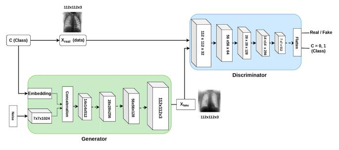
FIGURE 2. CovidGAN complete Architecture with generator and discriminator.
