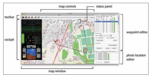
**Fig. 8:** *e-mo-tion* software panel, showing the map window, the waypoint editor and the photograph location editor (© senseFly LLC).
