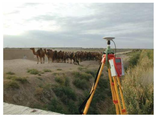
**Fig. 5:** The Lecia Global Positioning System (GPS) set up to establish a control point, on one of the road bridges near Ancient Merv, to geo-reference the IKONOS satellite image.
