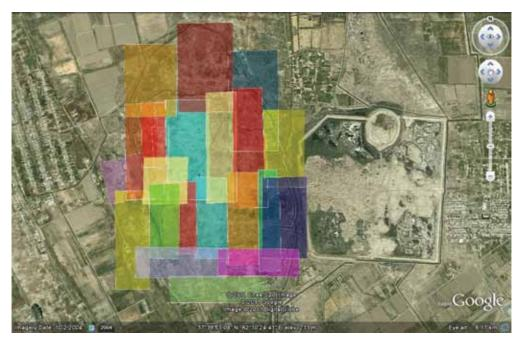
**Fig. 10:** Coverage of APs over Merv, with each coloured box representing a single flight. Note the larger area covered in the northern part of the survey, when flying at c.105m and capturing 4cm/pixel resolution images, as compared to the smaller survey grids to the south, at the 2cm/pixel resolution.
