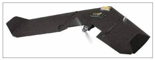
Fig. 6: The swinglet CAM UAV (© senseFly LLC).
