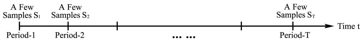
Figure S5: | Sampling periods (or time windows) and samples for the measured high-throughput data. The entire period is divided into [period-1 ,..., period- T ]. The interval between two consecutive periods (e.g., a month or a week) may be long, but the interval between two samples or sampling time points in each sampling period (e.g., a day or an hour) should be shorter so that the dynamical features can be reflected in the measured data. It each time period, we evaluate the composite index or DNB based on a few samples so as to check whether it is in the pre-disease state in this sampling period.
