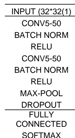
Figure 3: CNN Architecture with 2 convolutional and 2 max-pool layers.
