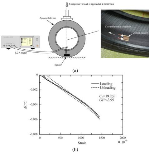
**Figure 4.** Self-sensor modeling of a steel wire belt in a radial tire as an electric resistor– condenser parallel circuit. The diagram is from Matsuzaki *et al.* [79] and is reprinted with permission from Elsevier.
