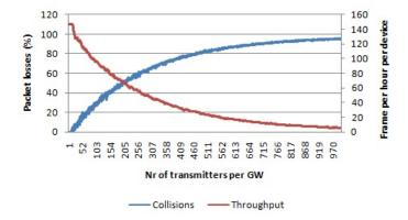
**Figure 12.** Percentage of packets lost due to collisions per number of transmitters per gateway using pure Aloha access. Average throughput per device. Payload size 20 bytes, single channel, multiple SFs.
