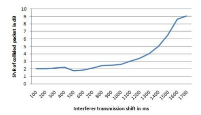
**Figure 3.** Average SNR value for received packets from the interfered transmitter for the first setting.
