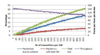
**Figure 9.** Percentage of packets lost due to collisions and the percentage of packets received with the wrong payload CRC per number of transmitters per gateway. Average throughput per device. Payload size 20 bytes, multiple channels, multiple SFs.
