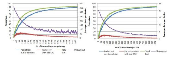
**Figure 6.** Percentage of packets lost due to collisions and percentage of packets received with the wrong payload CRC per number of transmitters per gateway. Average throughput per device. Single channel, single SF and payload size 20 bytes. (**left**) Using SF 7; (**right**) using SF 12.
