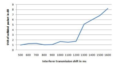
**Figure 4.** Average SNR value for received packets from the interfered transmitter for the first setting. For the first four shifts, there are no data since all the packets were lost.
