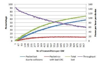
**Figure 7.** Percentage of packets lost due to collisions and percentage of packets received with the wrong payload CRC per number of transmitters per gateway. Average throughput per device. Payload size 20 bytes, single channel, multiple SFs.
