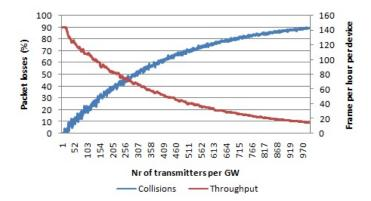
**Figure 14.** Percentage of packets lost due to collisions per number of transmitters per gateway using pure Aloha access. Average throughput per device. Payload size 20 bytes, multiple channels, multiple SFs.
