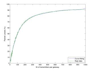
Figure 10. Curve fitting for single channel and SF 12.
