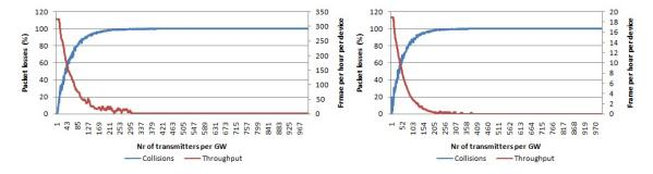
**Figure 11.** Percentage of packets lost due to collisions per number of transmitters per gateway using pure Aloha access. Average throughput per device. Single channel, single SF and payload size 20 bytes. (**left**) Using SF 7; (**right**) using SF 12.
