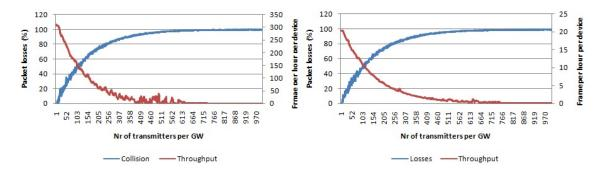
**Figure 13.** Percentage of packets lost due to collisions per number of transmitters per gateway using pure Aloha access. Average throughput per device. Multiple channels, single SF and payload size 20 bytes. (**left**) Using SF 7; (**right**) using SF 12.
