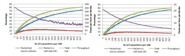
**Figure 8.** Percentage of packets lost due to collisions and the percentage of packets received with the wrong payload CRC per number of transmitters per gateway. Average throughput per device. Multiple channels, single SF and payload size 20 bytes. (**left**) Using SF 7; (**right**) using SF 12.
