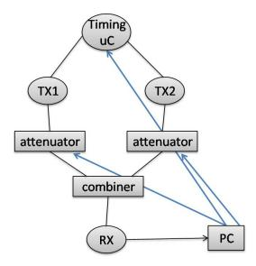
Figure 1. Controllable setup for measurements with real nodes.
