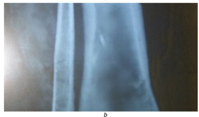
Fig. 3 Realistic phantom that mimics a cow's leg was prepared by using a bovine tibia and fibula bone section a Phantom's cross-section b Sagittal X-ray scan of the phantom
