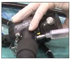
Figure 6: Syringe connected to suction nipple
