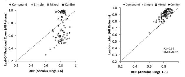
**Figure 3. Relationships between leaf-off and leaf-on lidar FC estimates and measured FC using digital hemispherical photography.** Axes are scaled differently to allow for best representation of the data. Regression relationships not shown for leaf-off lidar plot as data were not normally distributed precluding a statistically significant relationship. doi:10.1371/journal.pone.0054776.g003
