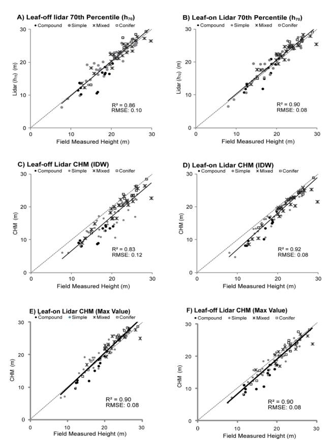
Figure 2. Regression relationships between measured average canopy height (H) and lidar values using: a) Leaf-off lidar 70<sup>th</sup> percentile; b) Leaf-on lidar 70<sup>th</sup> percentile; c) Leaf-off lidar IDW Interpolated CHM; d) Leaf-on lidar IDW Interpolated CHM; e) Leaf-off lidar Max Height CHM; f) Leaf-on lidar Max Height CHM. doi:10.1371/journal.pone.0054776.g002
