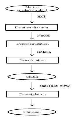
In chemical hydrolysis method, four main steps are involved in order to produce CTS from marine crustacean shell as depicted in Figure 2. They are (i) demineralization; (ii) deproteinization; (iii) discoloration and (iv) deacetylation. To produce 1 kg of 70% deacetylated CTS from shrimp shells, 6.3 kg of HCl and 1.8 kg of NaOH are required [8,9].
