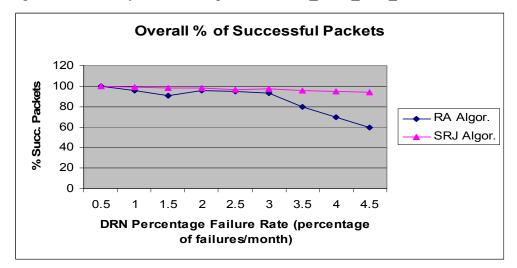
**Figure 12.** Simulation results for the hierarchical acoustic wireless sensor network. Percentage of successfully transmitted packets. NUM DRN PER DDN = 50.
