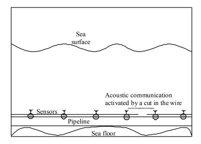
Figure 6. Integrated wired/acoustic wireless sensor network.
