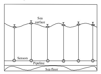
Figure 5. RF Wireless sensor network.
