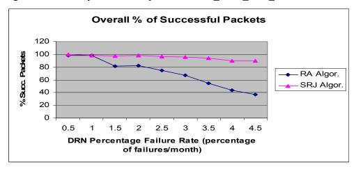
**Figure 13.** Simulation results for the hierarchical acoustic wireless sensor network. Percentage of successfully transmitted packets. NUM\_DRN\_PER\_DDN = 100.
