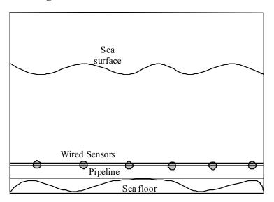
Figure 1. Underwater wired sensor network.
