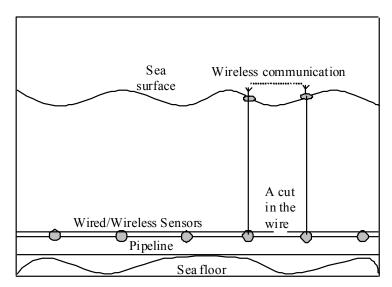
Figure 7. Integrated wired/RF wireless sensor network.
