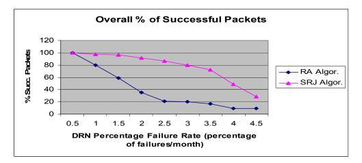
**Figure 14.** Simulation results for the hierarchical acoustic wireless sensor network. Percentage of successfully transmitted packets. NUM DRN PER DDN = 150.
