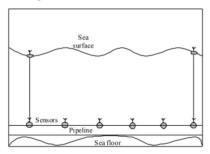
Figure 4. Underwater acoustic sensor network.
