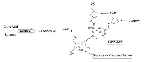
**Figure 5.** Proposed bridges and possible structures formed by the reaction citric acid with sucrose and with the furfural and hydroxymethyl furfural generated from sucrose by the citric acid treatment in sugar + citric acid adhesives [118].
