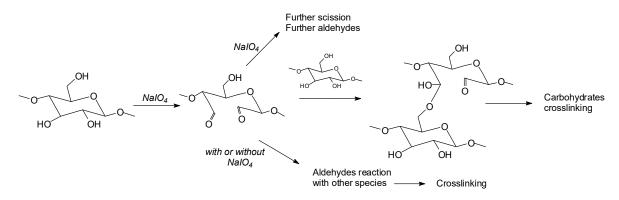
**Figure 2.** Specific oxidation of carbohydrates by sodium periodate leading to nontoxic and nonvolatile biosourced aldehydes and to different crosslinked products according to the conditions used [54].
