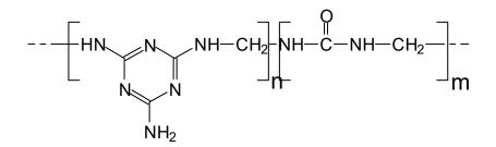
Scheme 2. Schematic representation of a MUF resin.
