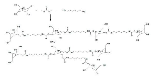
**Figure 3.** Schematic representation of the formation of non-isocyanate polyurethane (NIPU) oligomers from monosaccharides reacted with dimethyl carbonate and hexamethylene diamine. The two tetramers shown have been identified and are among the multitude of other NIPU oligomers identified [110].
