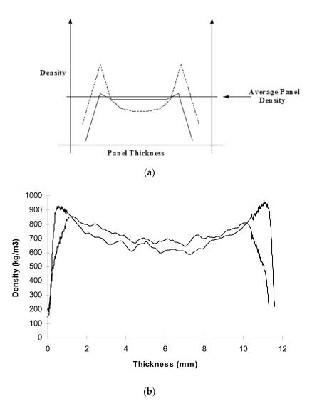
**Figure 1.** (**a**) Schematic, exaggerated representation of two different panel density profiles along the panel thickness leading to very different board properties; (**b**) an example of two real, different density profiles of two different wood particleboards [1].
