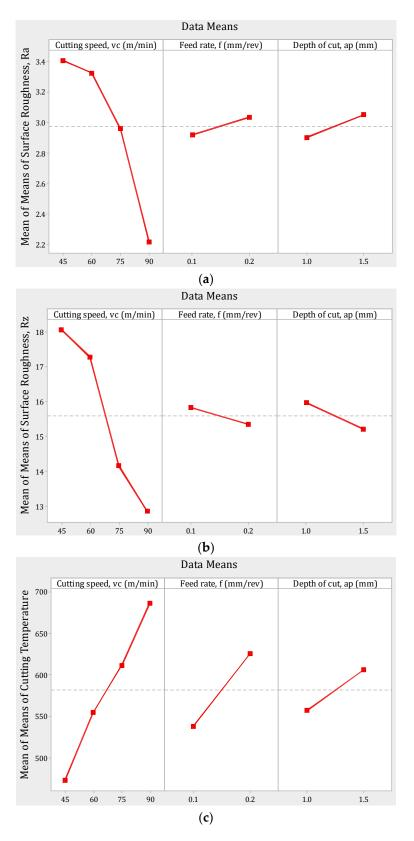
**Figure 3.** Effects of control factors on (**a**) mean of surface roughness,  $R_a$ , (**b**) mean of surface roughness,  $R_z$ , and (**c**) mean of cutting temperature.
