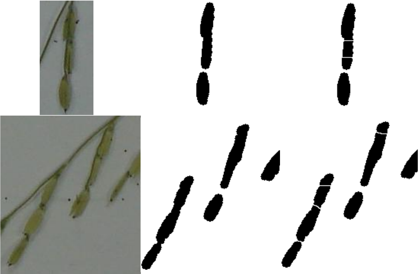
After applying the mathematical opening to the binary version of the sample with a disk of the grain size
