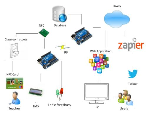
Immediately afterwards, the Arduino device connects to another Arduino (Master) by radio to identify the user accessing the classroom system. The system will use this ID to connect to the database and check whether it is a teacher and retrieve their name.
