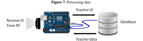
Initially, the receiver will connect to the network by using its Ethernet connection and prepare the necessary pin (pin 2) for receiving data via radio frequency. Once done, it will remain in standby until it receives the data.
