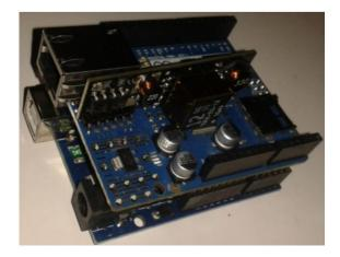
Figure 1. Arduino UNO and Ethernet shield.
