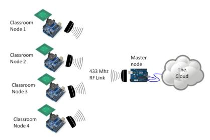
In more detail, the system would start working when trying to access a classroom (Figure 3), a process where an ID card would be used for this purpose. The user uses an NFC card reader connected to the Arduino device that shows a message on the LCD screen and one of the LEDs lights up, showing that the classroom is in use (red LED).
