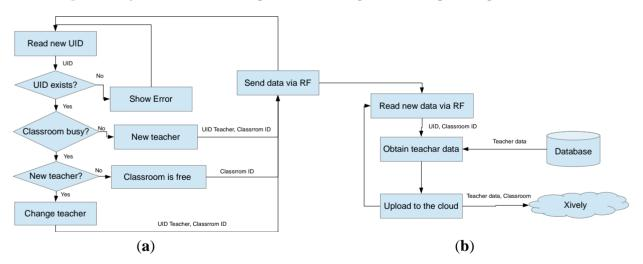
Figure 6a (see above) shows the reading process of cards. First the reader will read and identify two facts: ID and user name. In the NFC, and MiFare RFID technologies, the ID card is called UID. The UID is the first four bytes to be found in block 0 of sector 0. The other data should have been already saved. To record this information, keep in mind that each block is composed of sectors of 16 bytes. The write and read position is the address memory 4.
