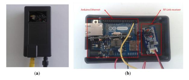
Figure 5. Master node hardware prototype: (a) outside (b) inside.
