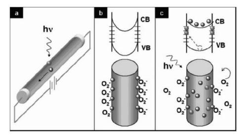
Figure 15. Photocurrent transport mechanism in a nanowire (reprinted from Reference [105]).
