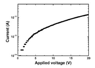
Normally the photoconductor is best suited for high photosensitivity, while a strong PPC was appeared. Due to the high resistivity of the epilayer, the photoconductor fabricated on an oxidized epilayer had a low dark current (1 pA) at 20 V. The dark *I-V* curve disclosed a space-charge-limited-current behavior, consistent with Ohmic contacts to a highly resistive material, as shown in Figure 10 [92].
