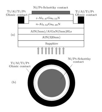
**Figure 4.** (a) Structure of Schottky-type back-illuminated photodetectors; (b) plan view of the contacts. (Reprinted from Reference [47]).
