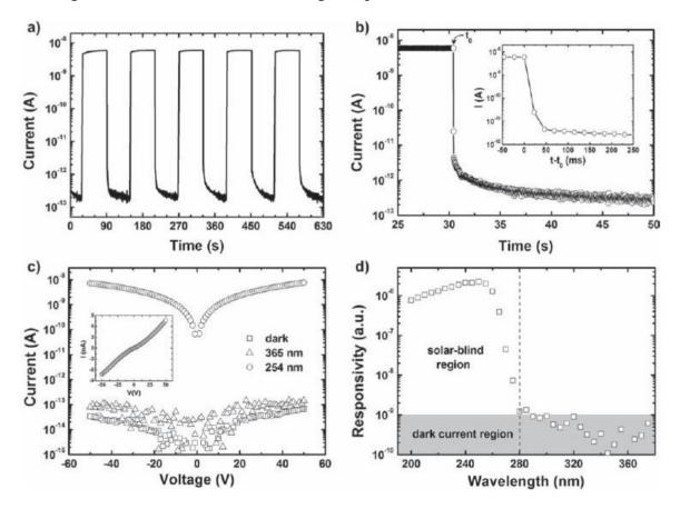
Li *et al.* reported the assembly of  $\beta$ -Ga<sub>2</sub>O<sub>3</sub> nanowires into high-performance solar-blind photodetectors by use of an efficient bridging method [117]. The photoresponse properties of the
