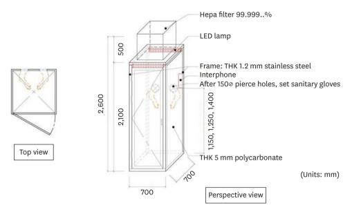
Fig. 1. Schematic blueprint of Safe Assessment and Fast Evaluation Technical booth of the H Plus Yangji Hospital.
