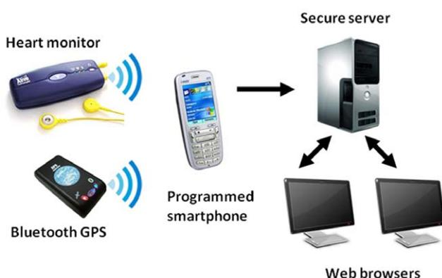
**Figure 2. Components of remote monitoring system.**
