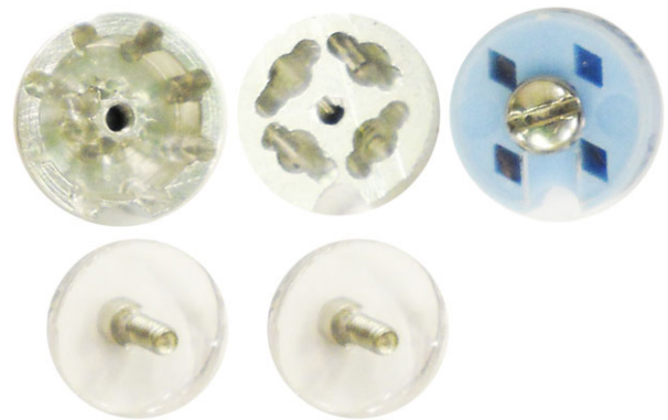
Fig. 1. The in house fabricated \text{Si}_3\text{N}_4 window storage box. This box has the same outer diameter as most standard cryo-TEM grid boxes (shown in the far right as a comparison) and fits most cryodevices such as FEI Vitrobot plunge freezer, Instec cryostorage mounting block, and Bionanoprobe sample transferring system. The box at the left has eight storage positions, whereas the box at the right has four storage positions. The window storage box is made of aluminium to minimize possible contamination from other high Z metals. It can be enclosed with a transparent lid secured by a stainless steel screw in the middle. The storage box allows windows to be vertically placed with predetermined orientation and to prevent fragile membranes from touching the aluminium wall during long-term storage and sample transportation.
