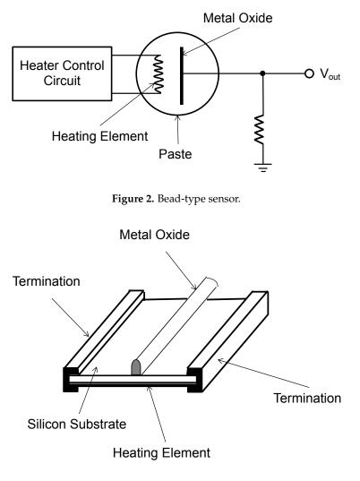
Figure 3. Chip-type Sensor.
