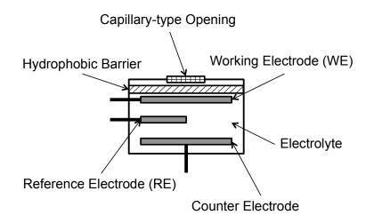
Figure 4. Basic Electrochemical Sensor.
