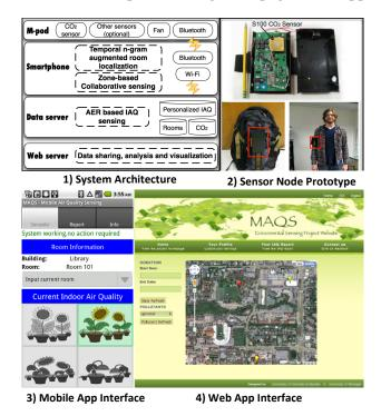
**Figure 9.** Example of the Community Sensor Network (CSN) system architecture and prototype. Figures are adapted from [109].
