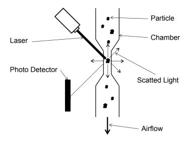
Figure 5. Basic Light Scatting Particle Counter.
