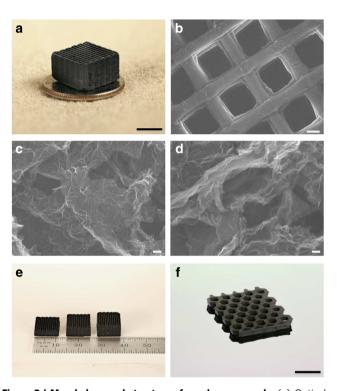
**Figure 2 | Morphology and structure of graphene aerogels. (a)** Optical image of a 3D printed graphene aerogel microlattice. SEM images of (b) a 3D printed graphene aerogel microlattice, (c) graphene aerogel without R-F after etching and (d) graphene aerogel with 4 wt% R-F after etching. Optical image of (e) 3D printed graphene aerogel microlattices with varying thickness and (f) a 3D printed graphene aerogel honeycomb. Scale bars, 5 mm (a), 200 μm (b), 100 nm (c,d), 1cm (f).
