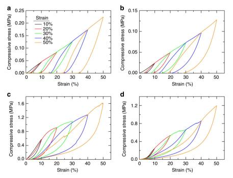
**Figure 4 | Compressive properties of graphene aerogels.** Stress-strain curves during loading-unloading cycles in sequence of increasing strain amplitude for (**a**) bulk graphene aerogel  $(31 \text{ mg cm}^{-3})$  and (**b**) 3D printed graphene aerogel microlattice  $(16 \text{ mg cm}^{-3})$  using the GO ink without R-F, (**c**) bulk graphene aerogel (123 mg cm<sup>-3</sup>) and (**d**) 3D printed graphene aerogel microlattice  $(53 \text{ mg cm}^{-3})$  using the GO ink with R-F.
