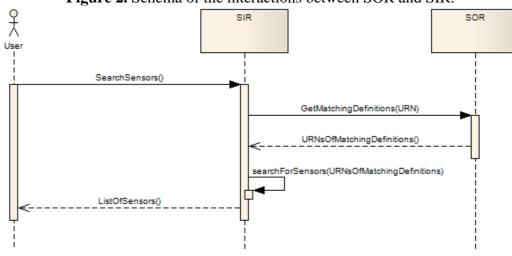
Figure 2. Schema of the interactions between SOR and SIR.
