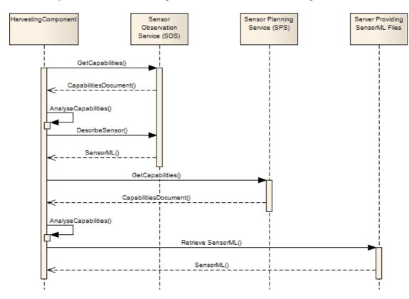
Figure 3. Schema showing of the SIR metadata harvesting mechanism.
