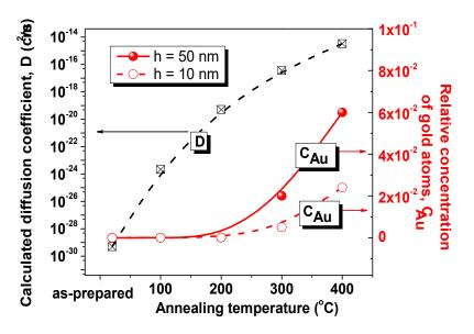
**Figure 5.** Effect of heat treatment temperature on gold atoms diffusion from a sublayer into the NiFe film: calculated values of the diffusion coefficient and relative concentration of gold atoms at a distance of 550 nm (or h = 50 nm) and 590 nm (or h = 10 nm) from the Au/NiFe interface.
