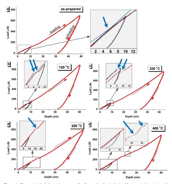
**Figure 4.** Characteristic deformation curves (loading-unloading) obtained by nanoindentation at the depth of 10 nm (black dots) and 50 nm (red dots) of the (**a**) as-prepared Au/NiFe nanostructured system and the same system after heat treatment with (**b**) 100 °C, (**c**) 200 °C, (**d**) 300 °C, and (**e**) 400 °C. The blue arrows indicate the moment the indenter passes through the interface of oxide and metal.
