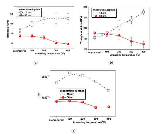
**Figure 3.** Mechanical properties of the Au/NiFe nanostructured system with indentation depth of 10 nm (black squares) and 50 nm (red circles) after heat treatment investigated using nanoindentation. (a) Dependence of the hardness, (b) Young's modulus, and (c) resistance to the elastoplastic deformation on the heat treatment temperature.
