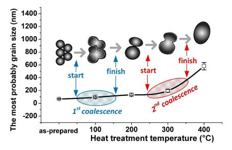
**Figure 2.** An increase in the most probable grain size upon heat treatment during two stages of coalescence. The most probable grain size was defined as the maximum of the function describing the grain size distribution in accordance with the Gauss law.
