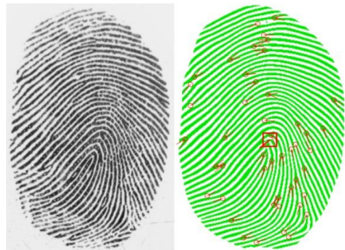
Fig. 2: Acquired and processed fingerprint image.
