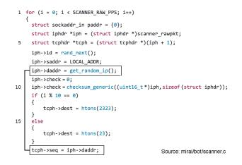
**Figure 2.** Mirai Scan Signature: The TCP scan packets are instantiated using the same value for the fields destination IP address and TCP Sequence number.
