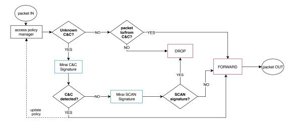
**Figure 6.** Mirai's execution flow: The malware initiates the propagation scan process and simultaneously contacts its C&C.
