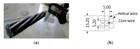
Figure 1. (a) Shape and (b) dimensions of PC strand.
